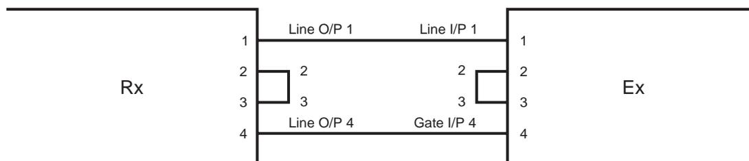
**Figure 13 D-Range Connections
