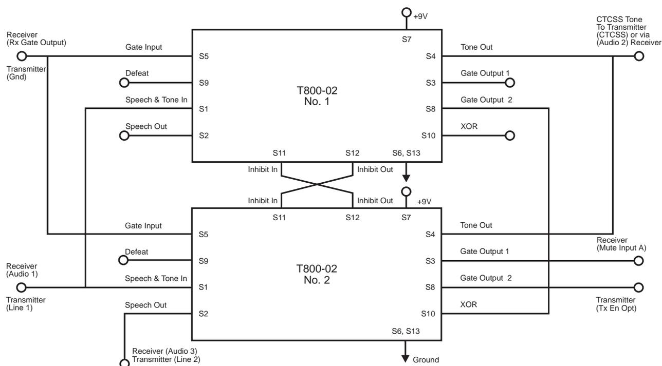
**Figure 10 Dual T800-02 Connection Details**
